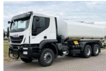
Cisterns tank: 24.000lt
